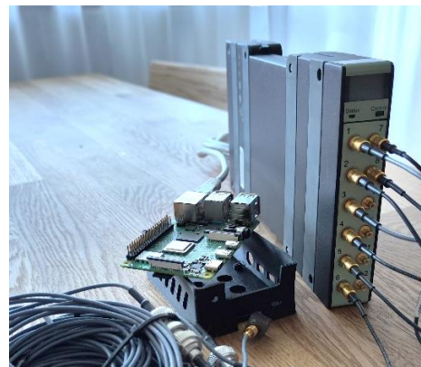
Figure 5. Left: 2 channels MCC172-based DAQ mounted on top of Raspberry Pi 5; Right: 12 channels B&K LAN-Xi-based DAQ and Raspberry Pi 4.
