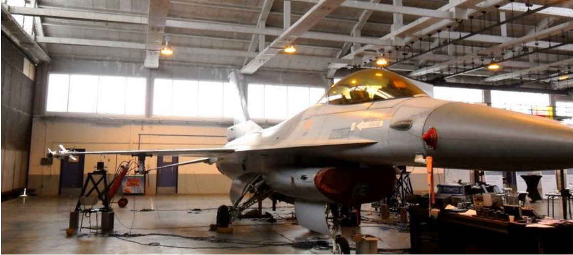
Figure 1. Ground Vibration Testing setup of the F-16 aircraft. Retrieved from [9].
